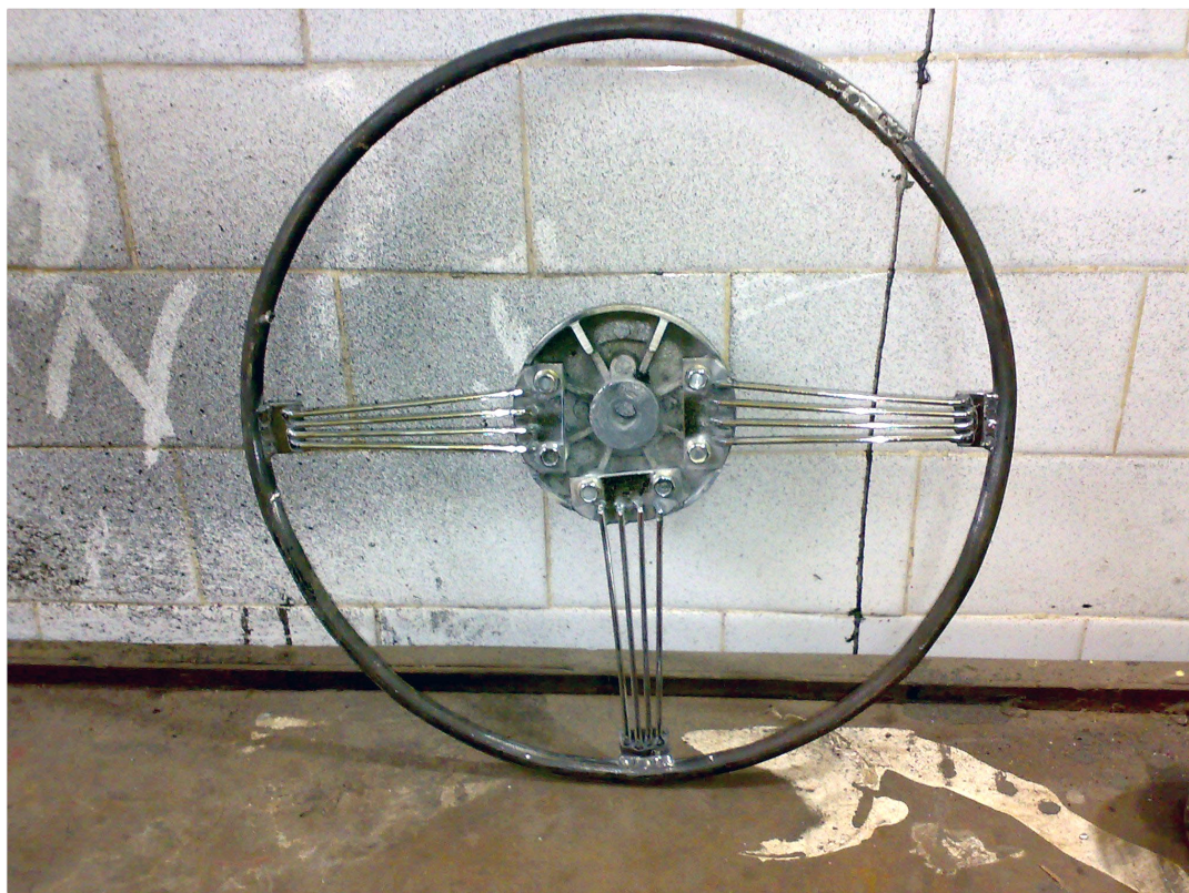
The Steering frame fitted with the spokes.
