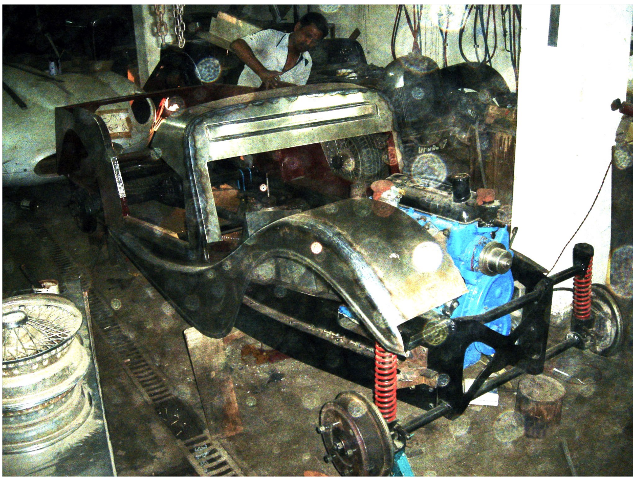
The fibreglass body being assembled.
