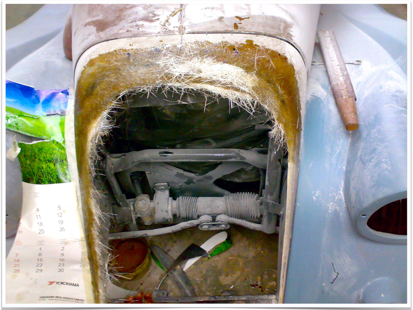
Fibreglass front end in the making.
