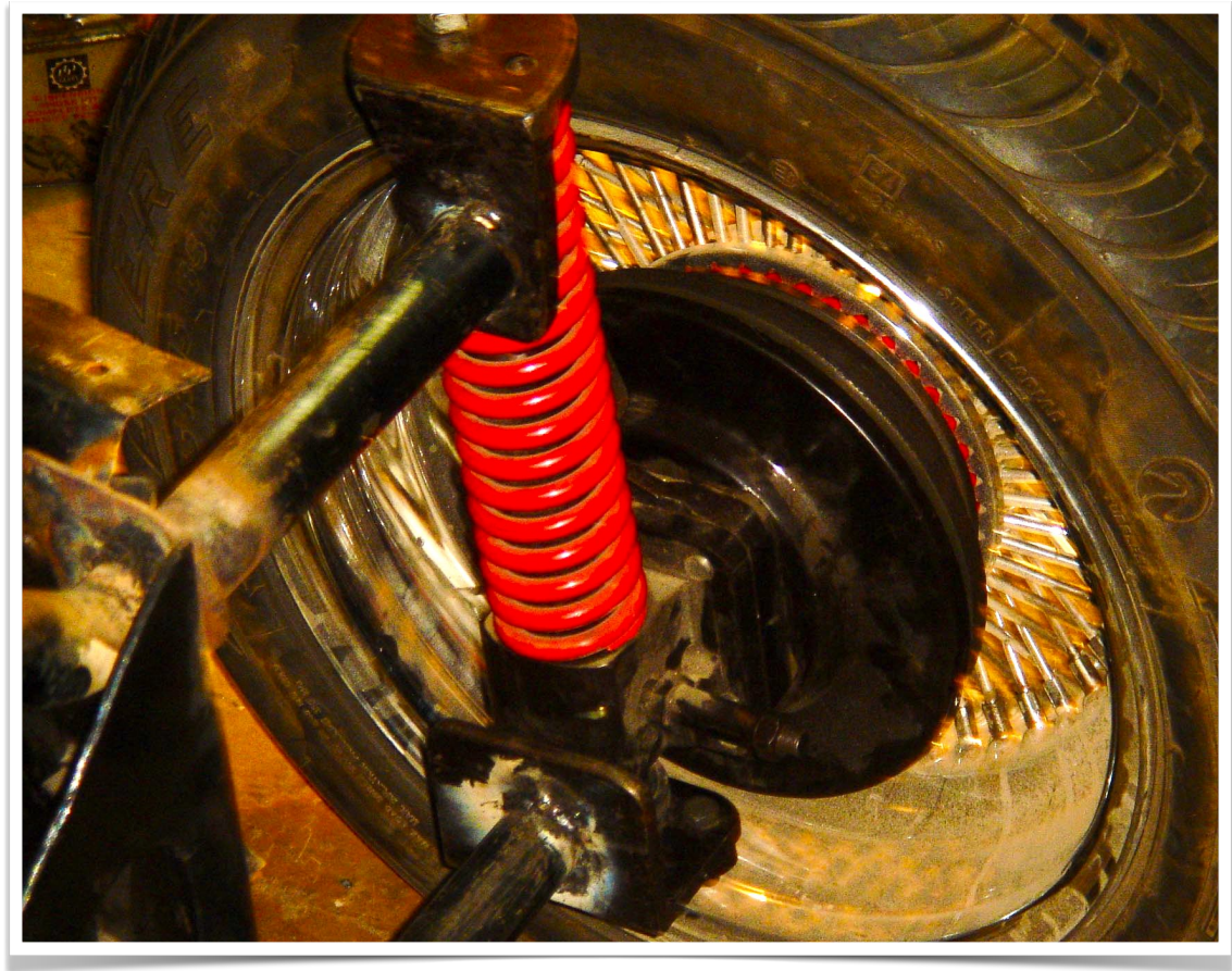
The front left suspension in place.
