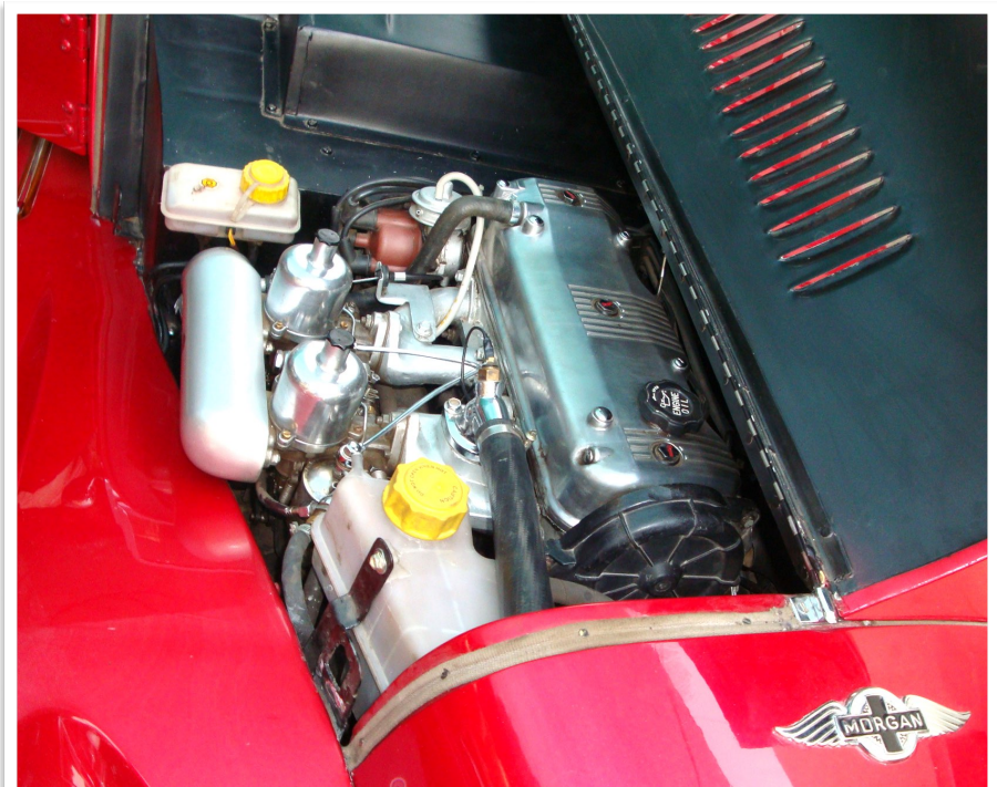
The twin SU Carburettors in place with the engine.
