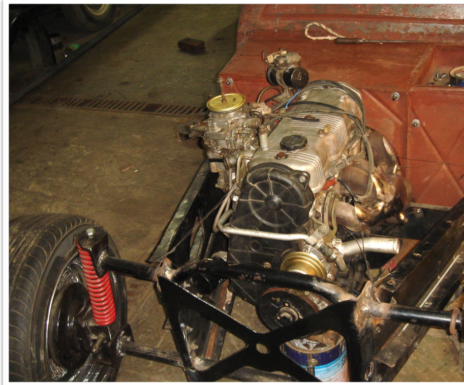
The 1800cc Isuzu engine mounted at the front end.
