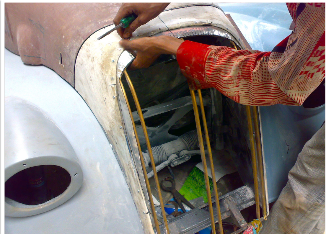
Grille Cowl in place and the grille leaves are being tested for fitting.
