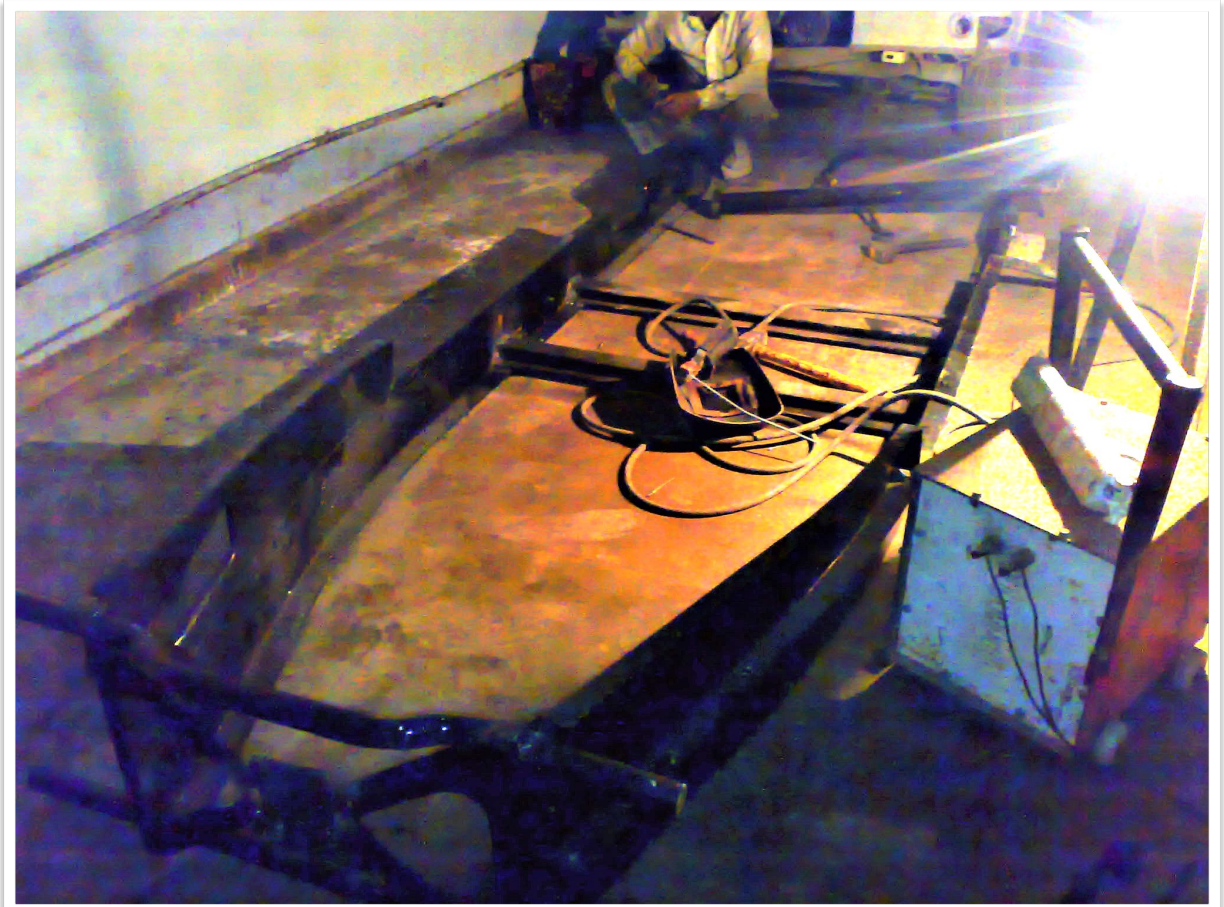
The assembled chassis rails of the Morgan.
